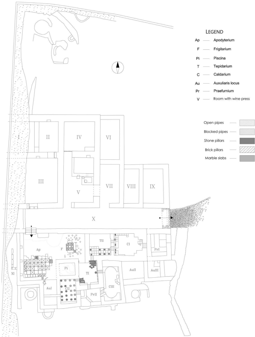
Figure 1.2 Ground plan of the bath house and the agricultural installation. Santorini (Thira), Kamari (©authors, Hellenic Ministry of Culture and Sports, Ephorate of Antiquities of Cyclades).
